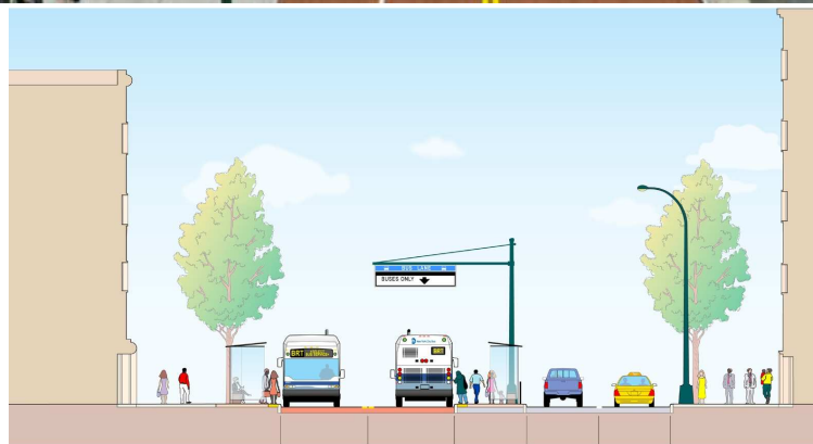
34th Street Cross Section: At Stations BRT Station BRT Lane BRT Lane BRT Station Travel Lane Travel Lane Sidewalk 11'-0" 11'-0" 10'-0" 10'-0" 10'-0" 6'-0" to 10' Feet 52'-0" Width of Roadway
